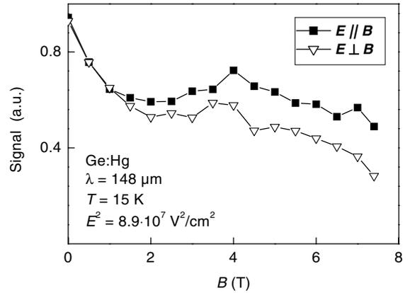
Figure 2: Photoconductive signal as a function of magnetic field strength for two  $E \perp B$  and  $E \parallel B$ .
