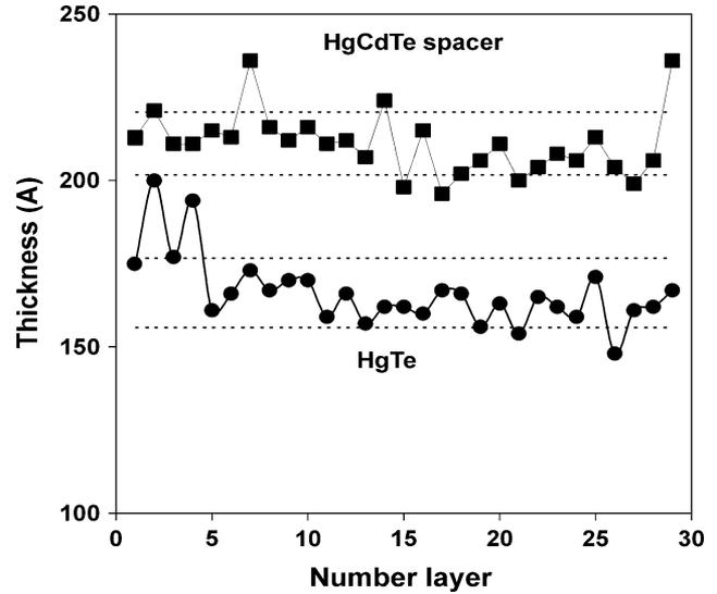
Fig. 6. HgTe and HgCdTe spacer layer in 30 HgTe QWs. *Solid lines*: average layer values; *dotted lines*: standard deviation. The average period of the structure is 37.7 nm ( $d_{\text{HgCdTe}} = 21.1$  and  $d_{\text{HgTe}} = 16.6$  nm).
