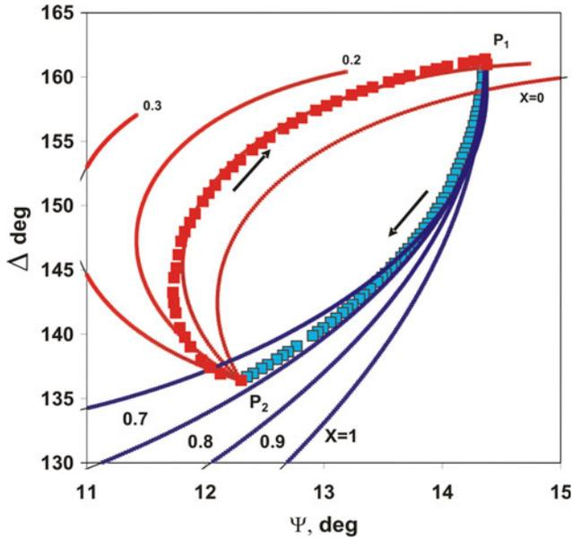
Fig. 5. Evolution of ellipsometric parameters  $\Delta$  and  $\psi$  during one cycle. *Dots*: experimental data; *solid line*: calculated data. Arrows indicate the direction of ellipsometric parameters  $\Delta$  and  $\psi$  during growth.  $P_1P_2$ : growth of HgCdTe spacer layer.  $P_2P_1$ : growth of HgTe layer.
