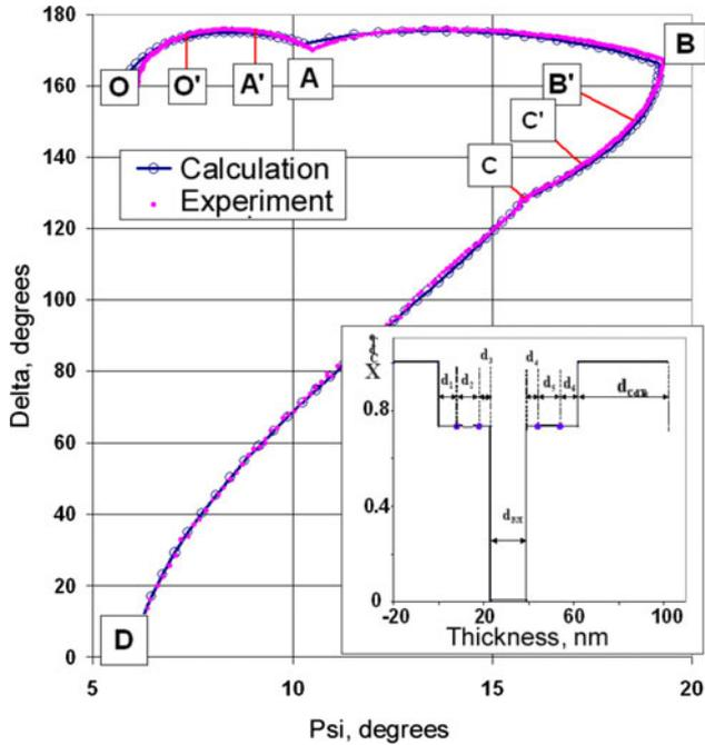
Fig. 2. Evolution of ellipsometric parameters  $\Delta$  and  $\psi$  during the growth of HgTe-based QWs. Points at curve knees (O–C) correspond to the initial stage of growth of the following QW layer. Dots: experimental data; solid line and circles (interval 1 nm): calculated data. Inset: MCT composition variation with thickness.
