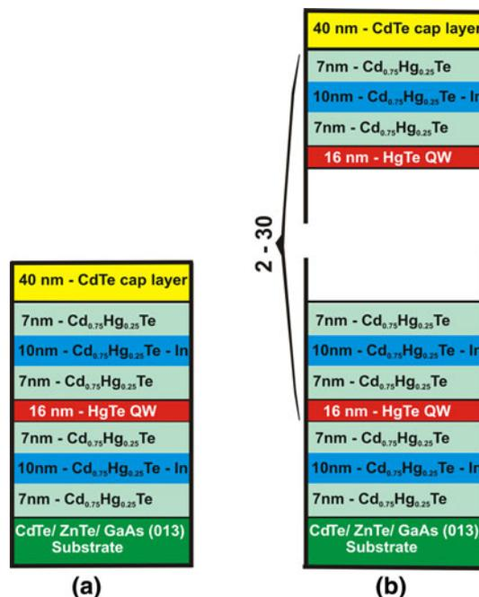
Fig. 1. Scheme of HgTe-based quantum wells: (a) single HgTe QW, and (b) multiple (2 to 30) HgTe QWs.
