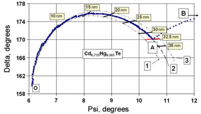
Fig. 3. Evolution of the ellipsometric parameters  $\Delta$  and  $\psi$  during wide-gap layer growth on the CdTe surface. Diamonds: experimental data. Lines 1–3: MCT composition calculations (1,  $x_{CdTe} = 0.75$ ; 2,  $x_{CdTe} = 0.735$ ; 3,  $x_{CdTe} = 0.72$ ). Lines transverse to OA correspond to equal thickness for different MCT compositions.
