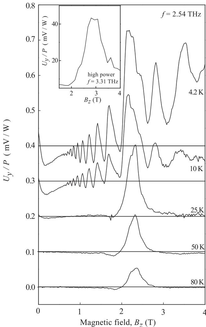
FIG. 3: Magnetic field dependence of  $U_y/P$  for linearly polarized radiation of  $f = 2.54$  THz and different temperatures  $T$ . The data for  $T < 80$  K are consistently shifted by  $+0.1$  mV/W for each step in temperature. Inset shows photovoltage resonance observed at 4.2 K under high power excitation of the pulse laser,  $f = 3.31$  THz. The signal  $U_y$  in the inset is normalized by the maximum detected signals,  $U_{y,max}$ .
