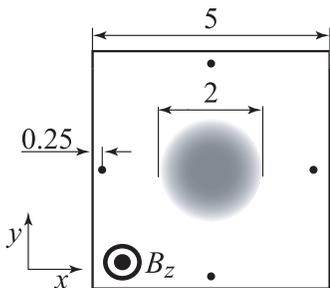
FIG. 6: Sample and contact dimensions in millimeters. Gray circle shows the laser spot located in the center of the sample. The spot has the Gaussian profile of about 2 mm diameter. Voltage drops  $U_x$  and  $U_y$  are measured between opposite contacts.
