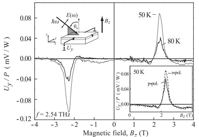
FIG. 1: Photosignal  $U_y$  normalized by the radiation power  $P$  excited by linearly polarized light ( $s$ -polarization) with  $f = 2.54$  THz as a function of the magnetic field  $B_z$ , incidence angle  $\theta_0 = 20^\circ$ . The left inset shows the experimental geometry. The right one presents the field dependences for  $s$ - and  $p$ -polarized radiation.
