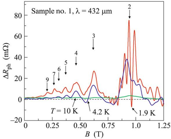
**Fig. 2.** Magnetic-field dependence of the photoresistance  $\Delta R_{\text{ph}}(B)$  for sample no. 1 under irradiation at the wavelength  $\lambda = 432 \mu\text{m}$  at temperatures of 1.9, 4.2, and 10 K. Arrows indicate the values of  $B$  corresponding to the cyclotron resonance harmonics.
