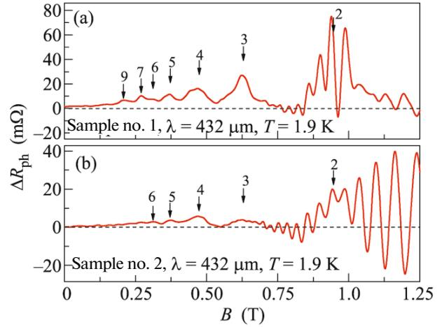
**Fig. 3.** Magnetic-field dependence of the photoresistance  $\Delta R_{\text{ph}}(B)$  for (a) sample no. 1 ( $N_s = 9.3 \times 10^{11} \text{ cm}^{-2}$ ,  $\mu = 1.45 \times 10^6 \text{ cm}^2/\text{V s}$ ) and (b) sample no. 2 ( $N_s = 9.3 \times 10^{11} \text{ cm}^{-2}$ ,  $\mu = 1.9 \times 10^6 \text{ cm}^2/\text{V s}$ ) at  $T = 1.9 \text{ K}$ .
