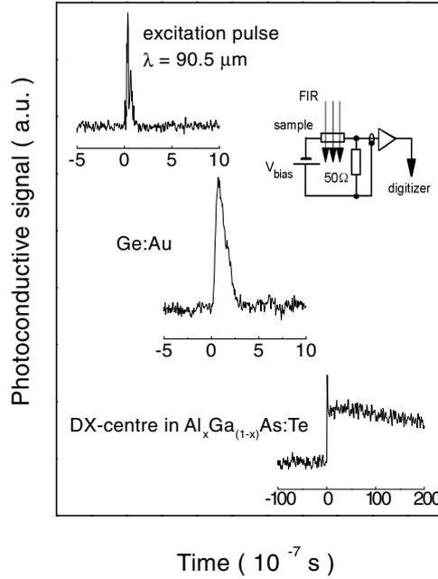
**Figure 10.** Oscillographic traces of the excitation pulse (top) at  $\lambda = 90.5 \mu\text{m}$  and of the photoconductive signals of Ge:Au (middle) and  $\text{Al}_x\text{Ga}_{1-x}\text{As:Te}$  (bottom, showing persistent photoconductivity at terahertz excitation!) The inset shows the measurement circuit.
